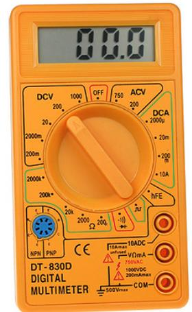
Devices that can be used to perform continuity tests include multimeters like the one to the right, which measure current and specialised continuity testers. In this unit each student will construct their very own continuity tester.
